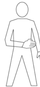
Raise arm, with fist clenched, horizontally in front of body, and then extend fingers. RELEASE BRAKE
