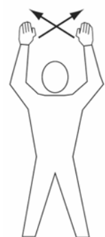
Waving arms overhead: EMERGENCY STOP
