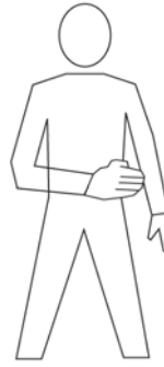
Raise arm, with fist clenched, horizontally in front of body, and then extend fingers. RELEASE BRAKE
